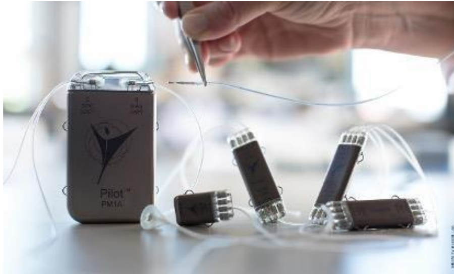
Figure 1: Illustration of the COSMIIC System (one PM, 4 RMs, multiple Network Cables and Electrodes)
